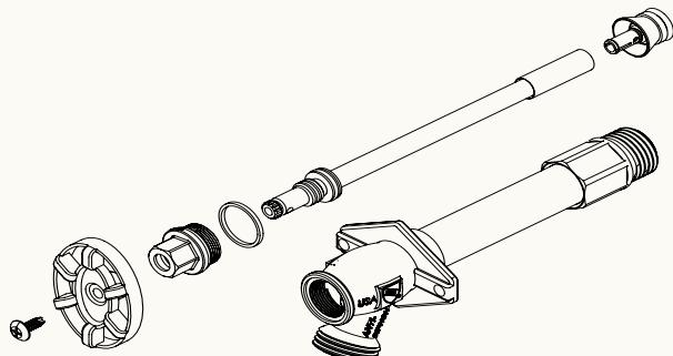
**WARNING:** Frost-Proof wall hydrants must be installed with a downward tilt toward the hose thread outlet AND the hose or other devices must be removed in cold and freezing weather. Failure to properly winterize a frost-proof wall hydrant can result in damage caused by freezing water and is not covered under warranty. For more information please visit our website at [www.arrowheadbrass.com](http://www.arrowheadbrass.com)
