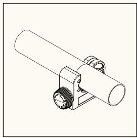
Step 1: make a clean, square cut with a pipe cutter and deburr the cut ends of the pipe to ensure a clean surface when inserting into the push-fitting.
