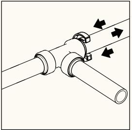
To disconnect Arrowhead Brass push-fittings place the push-fitting release tool against the push-fitting. Firmly push the release tool over the collar of the fitting (this will release the fitting). Pull the pipe out and remove the PEX insert if needed.
