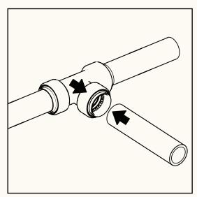
Step 3: insert the pipe into the Arrowhead Brass fitting and check the insertion depth mark.
