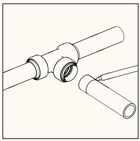
Step 2: mark the proper insertion depth on the pipe (see table below)
