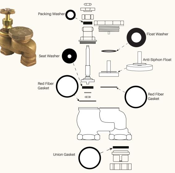
\*In order to rebuild, both the brass anti-siphon cap and the manual stem must be removed. \*\*Automatic valves will not have the manual flow control stem. Actuators must be removed to repair anti-siphon valve.
